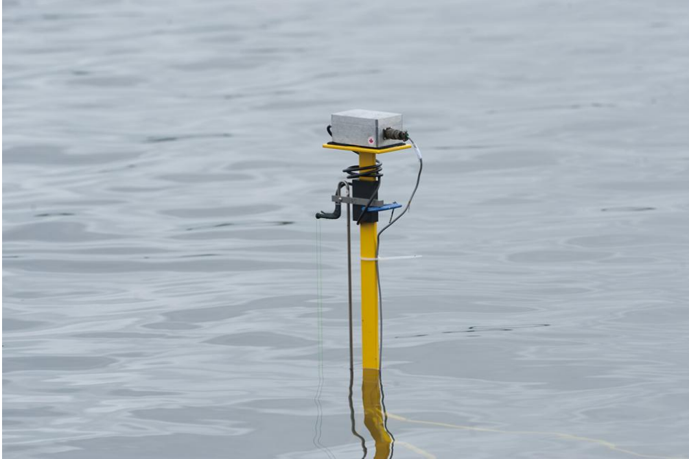
Figure 5. Station #2 with an Akamina AWP-24-2 capacitance wave probe.
