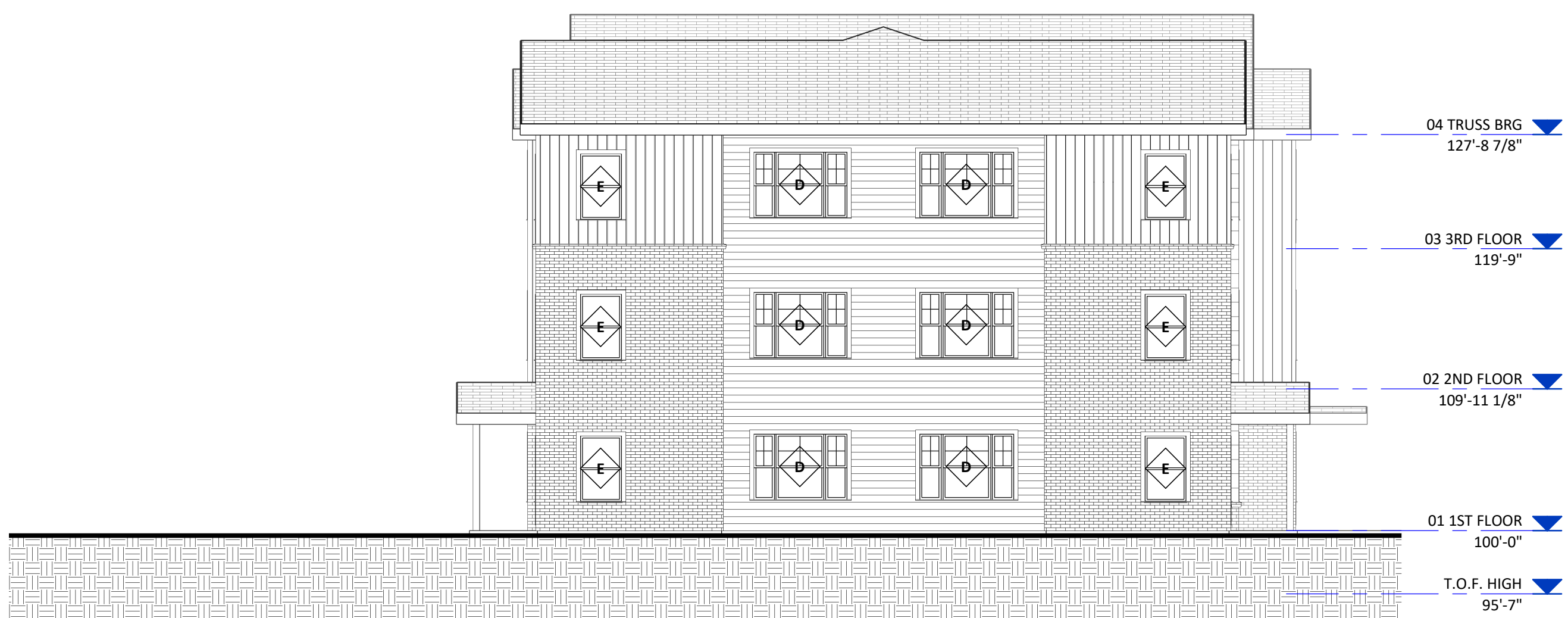
B4 BUILDING B SOUTH ELEVATION SCALE: 1/8" = 1'-0"
