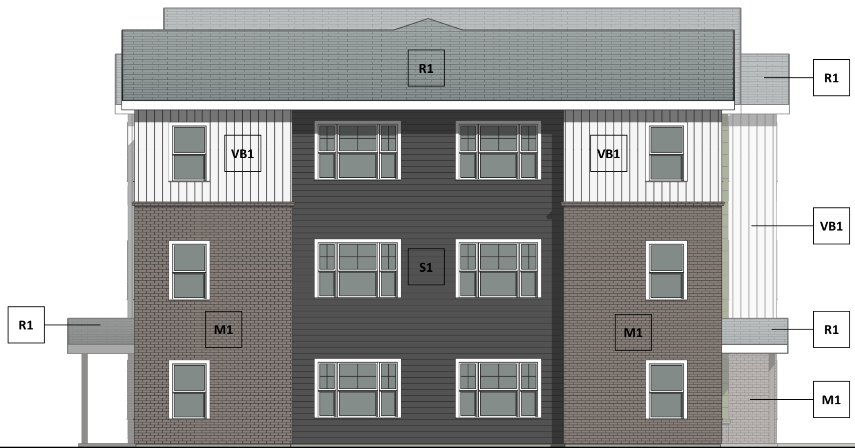
B5 BUILDING B SOUTH ELEVATION - COLOR SCALE: 1/8" = 1'-0"
