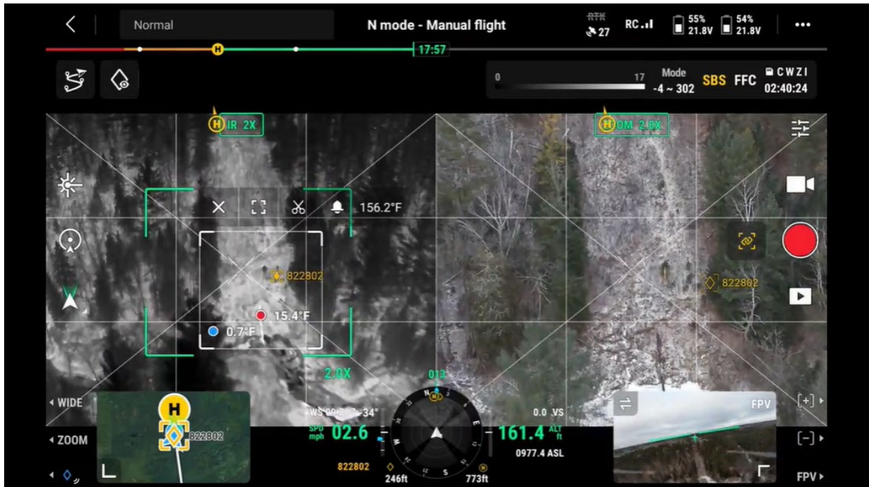
Figure 13. Screenshot from a drone flight over an exposed natural gas pipeline on Reservation, showing both an aerial and white-hot thermal image side-by-side. Thermal imaging is showing a temperature difference between the pipeline and the surrounding area.
